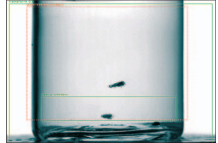
Particle detected with light transmission method
